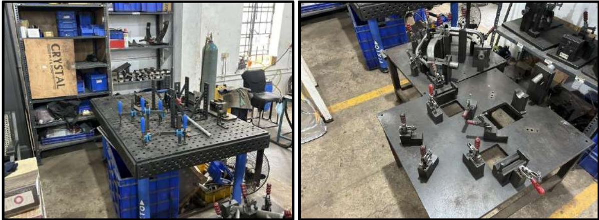
Pictures 11 & 12: Welding fixtures
